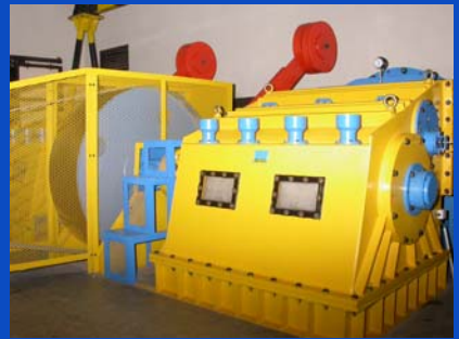
X-flow Turbine T-15 D500 head: 5 – 100 meter power: 50 – 600 kW
