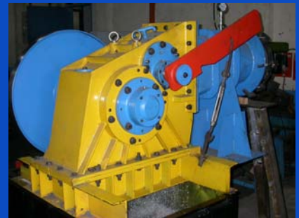
Nam Ka, Laos, project for entec X-flow T-14 -15 kW-Solar-Grid 2006
