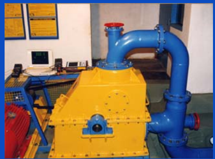
Pelton Turbine head: 70 – 300 meter power: 50 – 1000 kW
