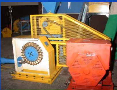
Peltric Turbine head: 15 – 100 meter power: 1 – 30 kW
