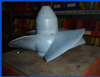
Propeller S-Turbine head: 2 – 13 meter power: 10 - 150 kW
