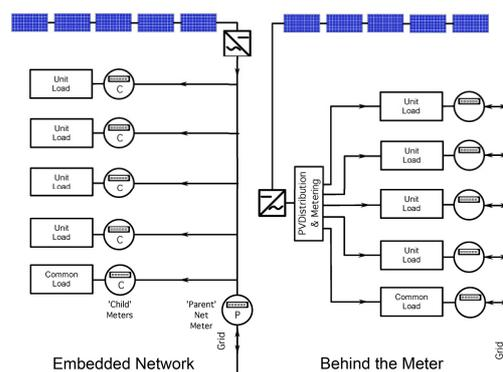
Fig. 1. Embedded Network and Behind the Meter Arrangements
