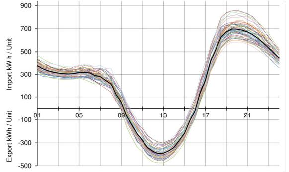
Fig. 2 Average daily load profile for 50 VBs with PV = 1.74 kW<sub>p</sub>/unit
