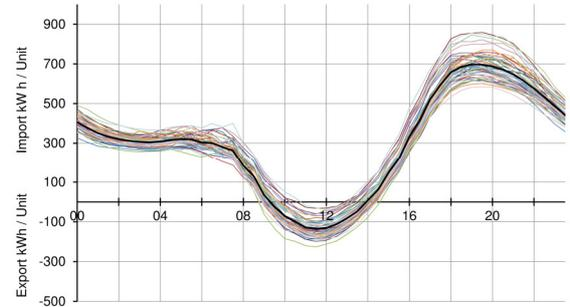
Fig. 3 Average daily load profile for 50 VBs with PV = 1.06 kW<sub>p</sub>/unit
