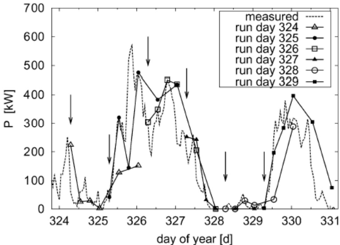
**Figure 3. Comparison of measured and predicted output of a wind turbine (Focken et al, 2002). The downward pointing arrows show the first (6 hour) forecast in each set of 6, 12, 18, 24, 36 and 48-hour forecasts. The 6 and 12-hour forecasts are always accurate in this example.**
