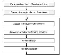
Figure 1. General procedure for evolutionary programming.
