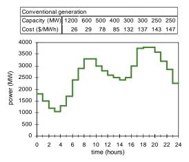
Figure 3. Power system load profile and thermal generating plant capacity and operating costs.
