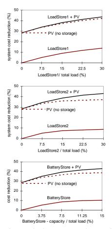
Figure 8. Reduction in system operating costs for increasing storage penetrations without PV, and with 70% PV penetration. The dotted line represents what cost reductions might be expected from PV and storage if no synergies existed.
