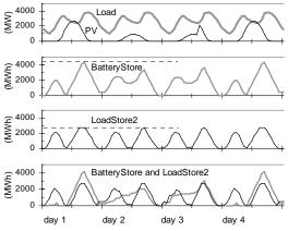
Figure 9. Simulated operation of power system as for Figure 7, but now including optimal storage operation when both storages are present.
