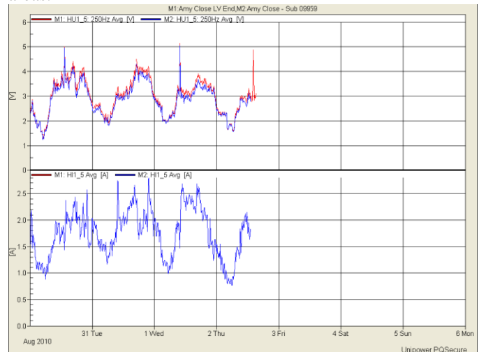
Fig 10. Voltage and current 5th harmonic values. Note the rise (especially in current harmonics) between the date lines which is when the PV is generating
