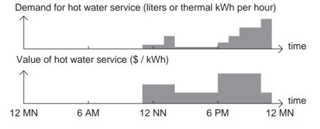
Figure 2: An example of how to use the proposed energy service model to describe the demand for and benefit of hot water service in a restaurant.
