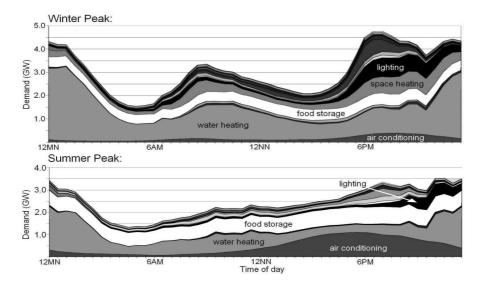
Figure 1: Total peak electricity demand of the residential sector in New South Wales, Australia, broken down by application, in June 2002 and January 2003. These are edited versions of the original figures in [Consultant Pty Limited, 2004].
