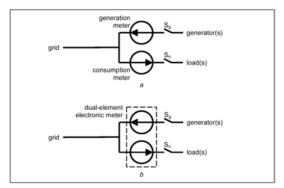
**Metering schemes 3a and 3b:** Generation and gross consumption are separately metered by (*a*) two unidirectional meters, one on the generator leg and one on the load leg, or (*b*) a dualelement electronic meter with one element on the generator leg and the other on the load leg. In some instances, the normal supply main switch is placed on the grid side of the common point.
