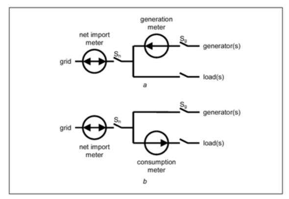
**Metering schemes 4a and 4b:** One bidirectional meter is used to measure net imports and a separate unidirectional meter is used to measure (*a*) generation or (*b*) gross consumption.
