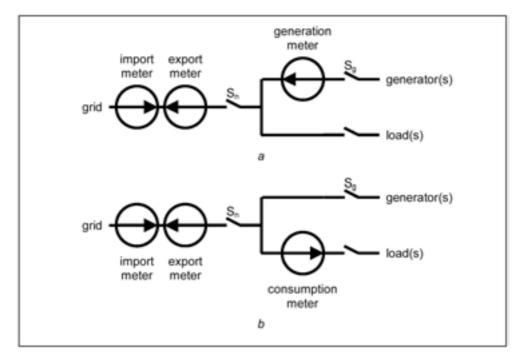
**Metering schemes 5a and 5b:** One unidirectional meter is used to measure gross imports, another is used to measure exports and a third is used to measure (*a*) generation or (*b*) gross consumption.
