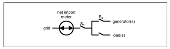
**Metering scheme 1:** A single bidirectional meter measures net flow of electrical energy between the grid and customer.
