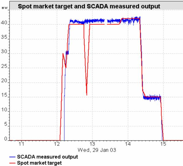
Fig. 2. Graph illustrating market targets and actual SCADA generation for a generator in the Australian NEM [20]
