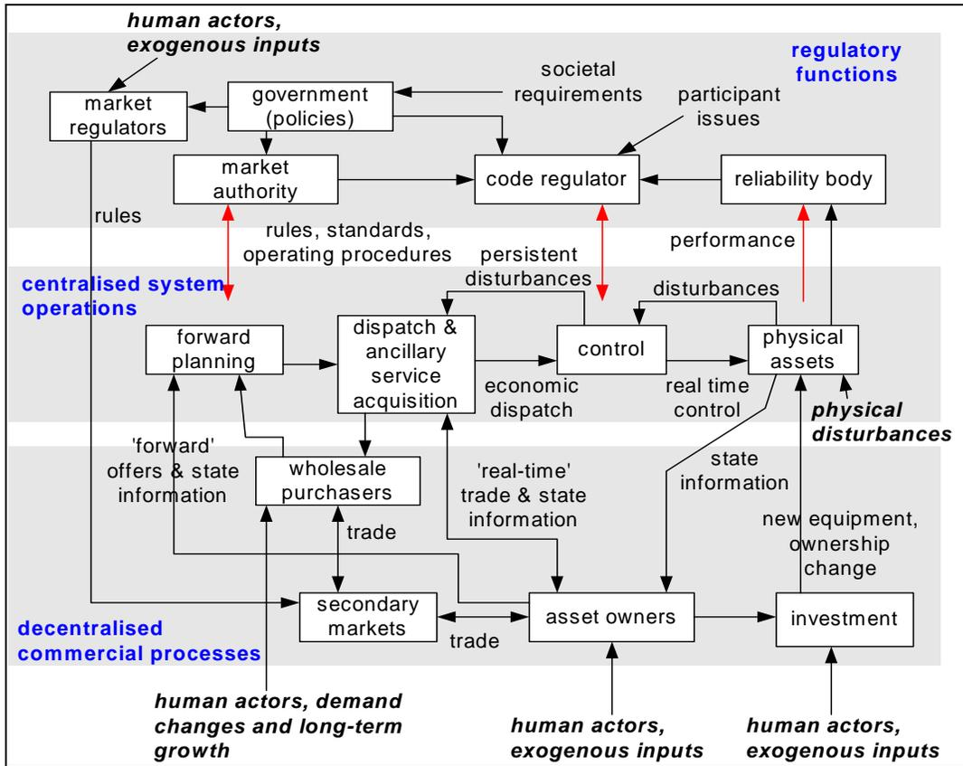
Fig 1. Processes and information flow diagram for a restructured electricity industry.
